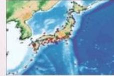
JMA operates around 80 tide gauges and also collects real-time sea level data from gauges operated by other organizations. The Agency further uses 18 GPS buoys and 38 offshore-water-pressure gauges managed in conjunction with other organizations for Tsunami Information.
